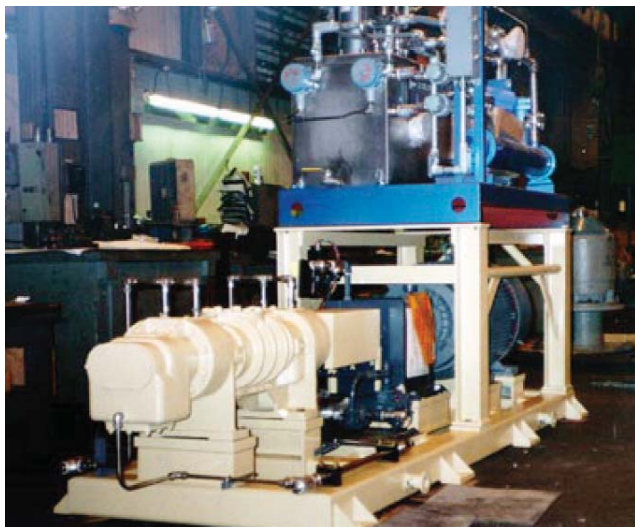
Figure 3 Twin-screw Naphtha Main Gas Turbine Fuel Pump
